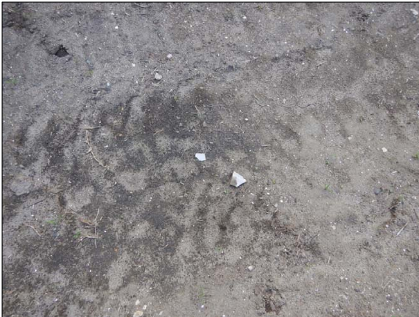
Figure 14: Evidence of Fill and possible ACM fragment
