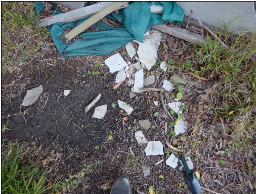
Figure 10: Fibro fragments around weatherboard house
